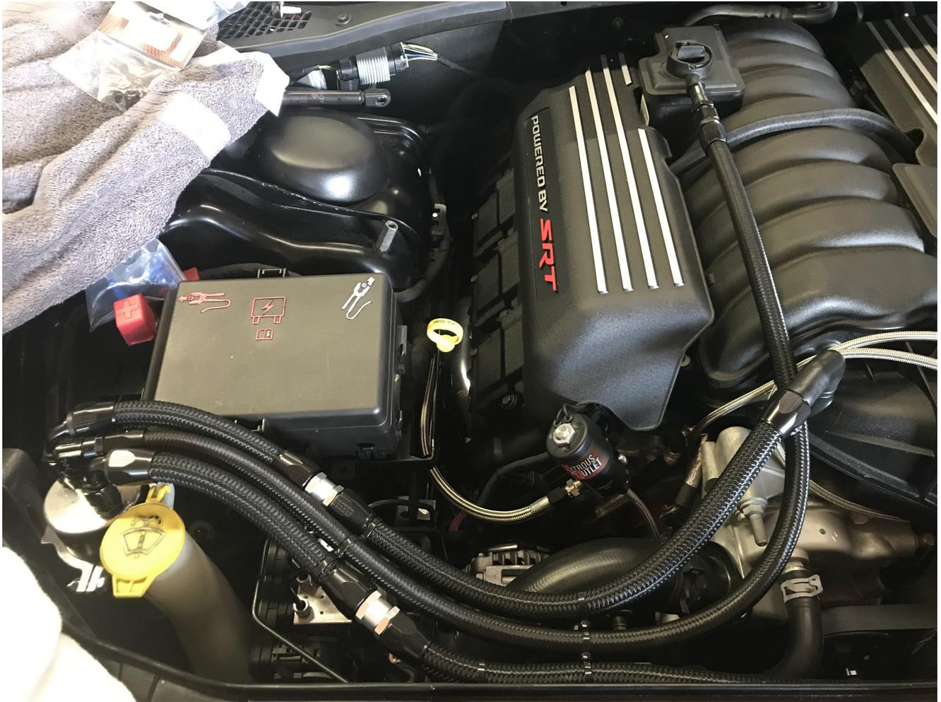
Here you can see one of the mount locations. It can also be mounted off the stud on the water pump. Center of can, no checkvalves, goes to the crankcase outlet as shown.
