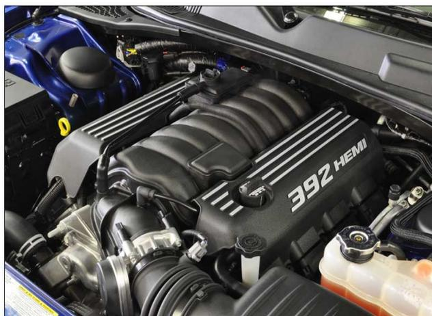
Above right, this fresh air is then drawn past the rocker arms and down through the crankcase and up and out the passenger side flushing and making up for the foul contaminated vapors being evacuated (sucked out) the factory separator on the passenger side. Next we will show mounting options and routing the can itself.
